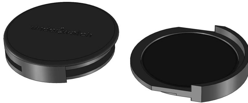
Figure 7-4: CAD model of a 3-D printed mock-up of the underwatch fall detector used to demonstrate the battery drawer. The upper face in this picture is the side that contains the pulse sensor, placed against the skin. The battery drawer is shown removed on the right hand side.
