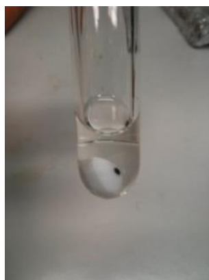
Figure 17. Bi-phasic reactor used for the solvent free epoxidation of limonene
