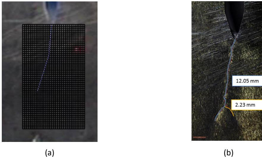
Figure 5.11: (a) grid of data acquisition points - LDV scan region; (b) fatigue crack microscope inspection (front surface).
