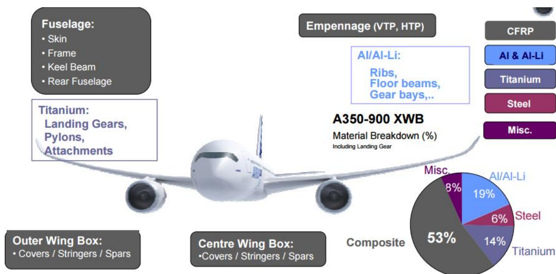
Figure 1.1: Airbus A350XWB materials used by weight; reproduced from [1].
