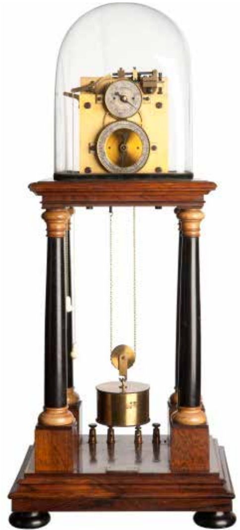
A Hipp chronoscope, as used in Wundt's psychophysics experiments
