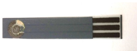
Figure 4.15: SPE with dry picric acid on the working electrode. The picric acid crystallizes when dry.
