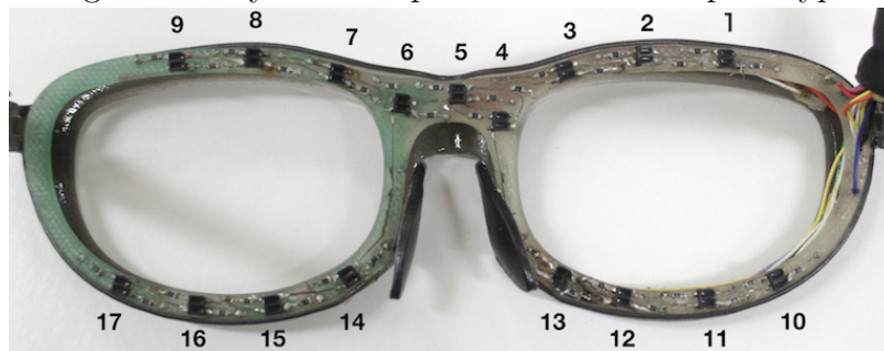
Figure 3-5: The placement of photo-reflective sensors for the first prototype
