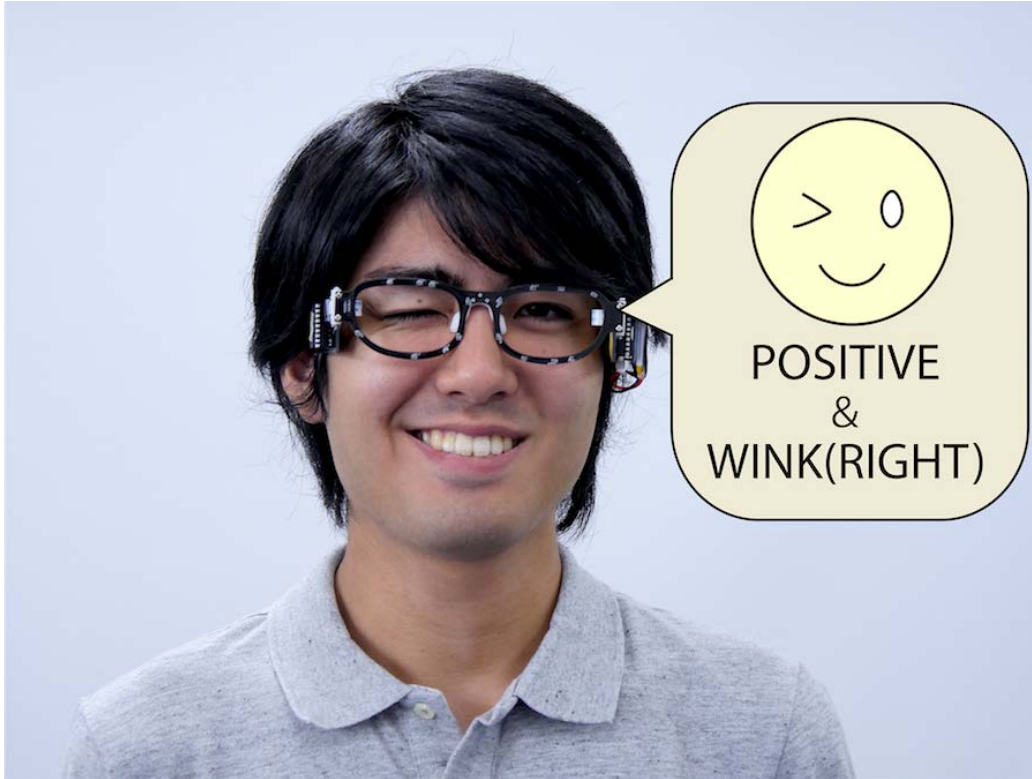
Figure 6-1: The user wears the prototype. The system can detect facial expression and eye gestures
