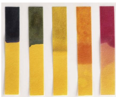
Figure 1-1. The colorimetric behavior of pH indicators in different conditions.
