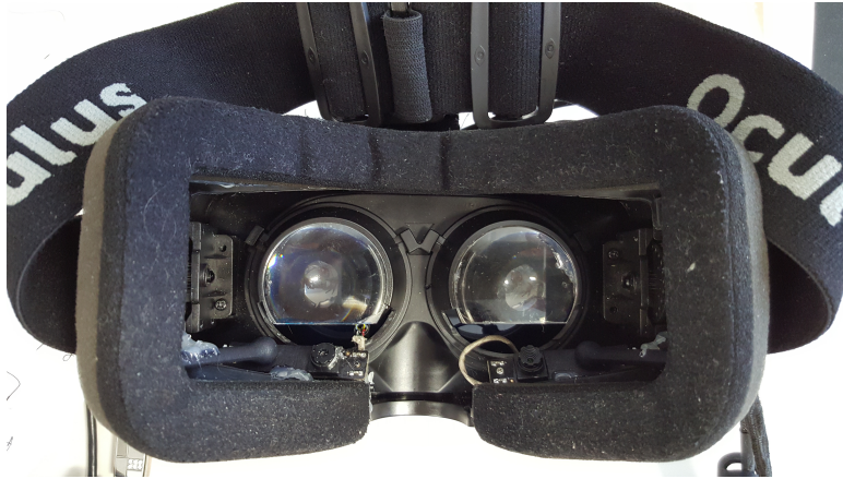
Figure 4.36: Placement of the eye trackers in DK2
