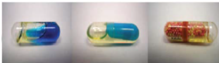
Figure 4.3 . Examples of various fills of capsule-in-capsule technology: liquid/liquid; liquid/semi-solid; liquid/beads (Rao et al. , 2013)
