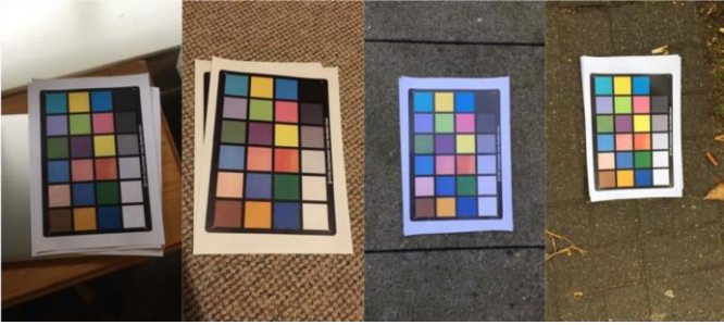
Fig. 3. (A) Two example images in the first dataset. Two identical 9-patch color charts appear in different positions in every image. The illumination is nonuniform with varied colors. (B) Examples of images in the second dataset taken under dynamic illumination conditions. A uniform illuminated color chart appears in every image in the dataset.
