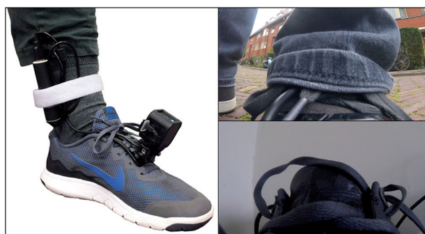
Fig. 2. Left: Study setup with camera secured to the shoelace of the shoe and focused on the lower leg. A powerbank, attached to the ankle with Velcro, provided the camera with sufficient power. Right: A sample from the camera data during use (top) and non-use (bottom) of the footwear.
