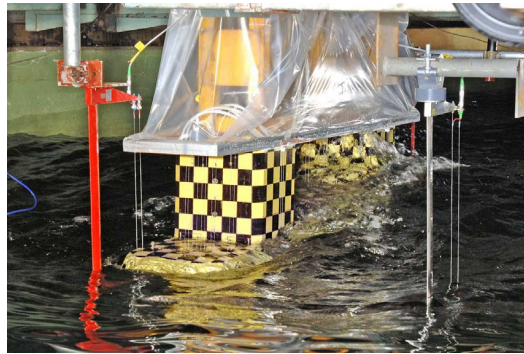
Figure 1: Photo snapshot of wave impact in the semi-submersible model experiment performed at MARIN, courtesy: “SafeFLOW” project
