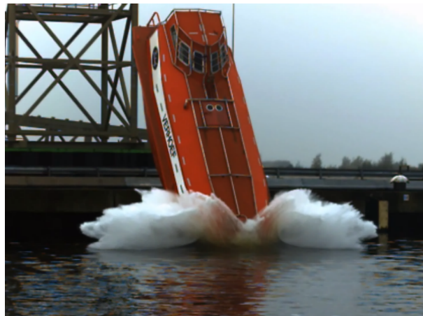
Figure 1: Drop test with free-fall lifeboat (from: www.verhoef.eu )
