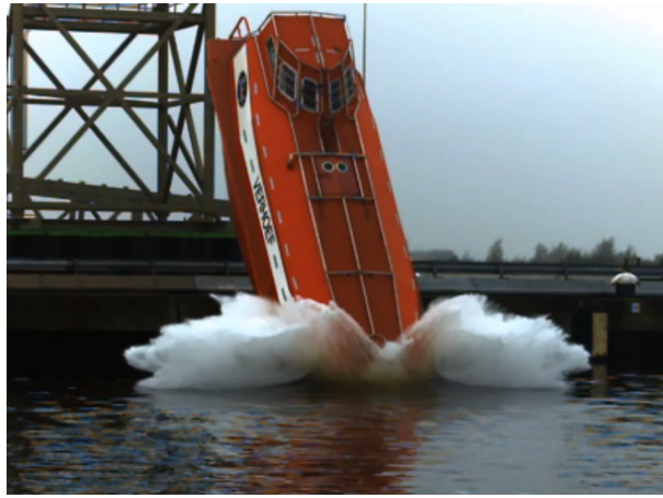
Figure 1: Drop test with free-fall lifeboat (from: www.verhoef.eu )
