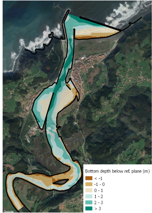
Figure 2: Bottom depth below ref. plane (m).
