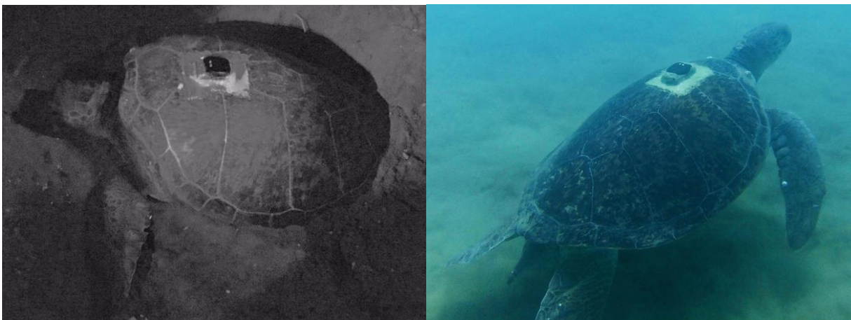
Figure 4.14: PitStop GPS Lite Tag, deployed on a green sea turtle in Cyprus. Photos taken by Julia Haywood from University of Exeter.
