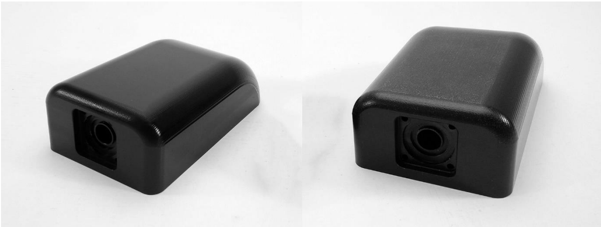
Figure 6.25: Polyoxymethylene (POM) and polyethylene (PE) enclosure shells that were tested for high-pressure resistance.
