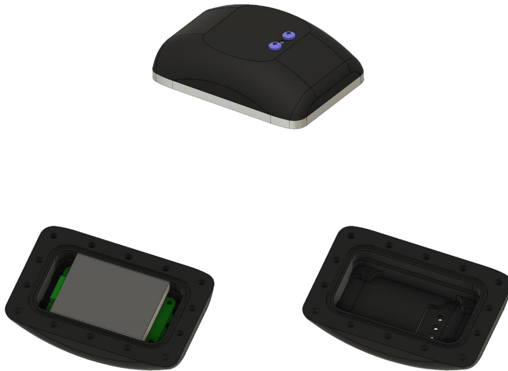
Figure 4.12: A few screenshots of the PitStop GPS Lite Tag in Autodesk Fusion 360. On the top is the assembled tag and on the bottom the inside of the enclosure with the mounting points for the electronic modules.
