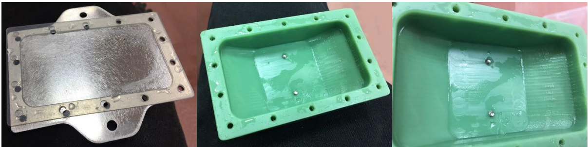
Figure 6.11: Oilamid enclosure shell with silicone gasket was the wettest of all cases with a silicon gasket whit big wet spots inside.
