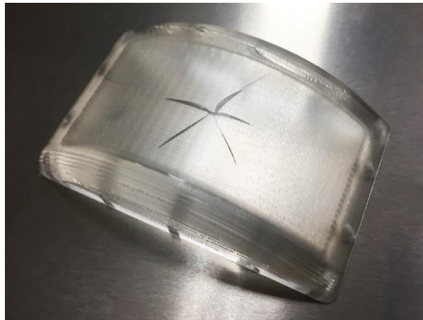
Figure 6.2: Acrylic enclosure shell tested broke without any load at 40° angle.
