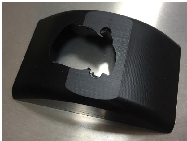
Figure 6.3: Polyoxymethylene (POM) enclosure shell tested broke after a series of tries under 9,025 kg of load at 67° angle.
