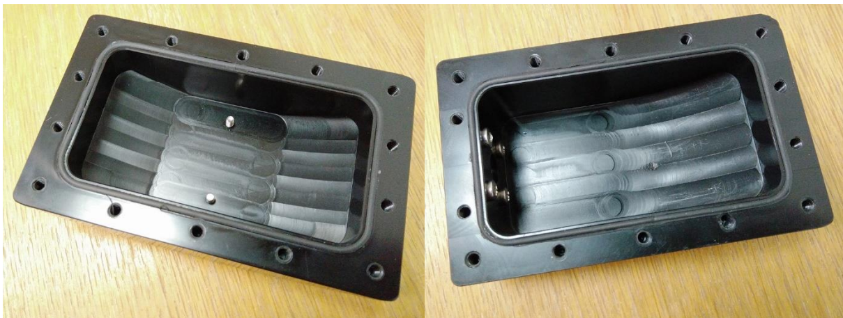
Figure 6.16: Both PitStop GPS Tag and PitStop Camera Tag enclosures stayed completely dry at 10, 25 and even 50 bar.
