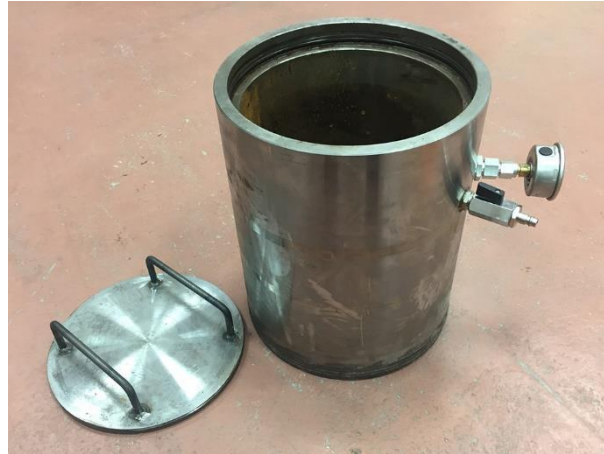
Figure 6.6: Pressure container, used for sealing tests.
