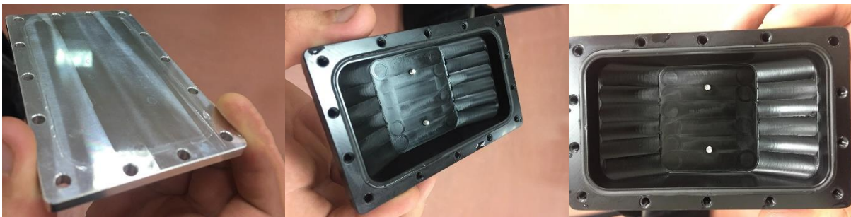
Figure 6.14: The second test of polyoxymethylene (POM) enclosure shell with rubber O-ring string, this time with two self-sealing screws for the salt water switch on the top of the case. The enclosure stayed completely dry even on the second try with the self-sealing screws.
