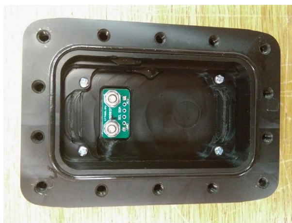
Figure 6.18: The turtle tag enclosures with the depth of O-ring groove of more than 1,40 mm had a few problems with small leaks in certain cases.
