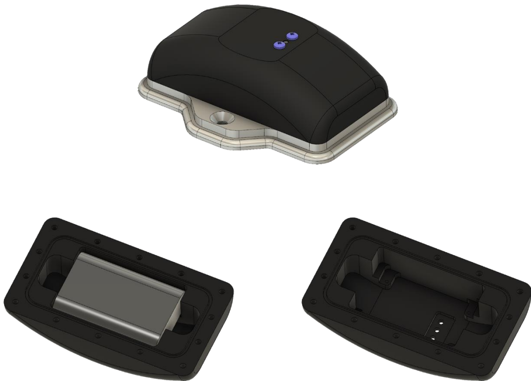
Figure 4.7: A few screenshots of the final version of PitStop GPS Tag in Autodesk Fusion 360.
