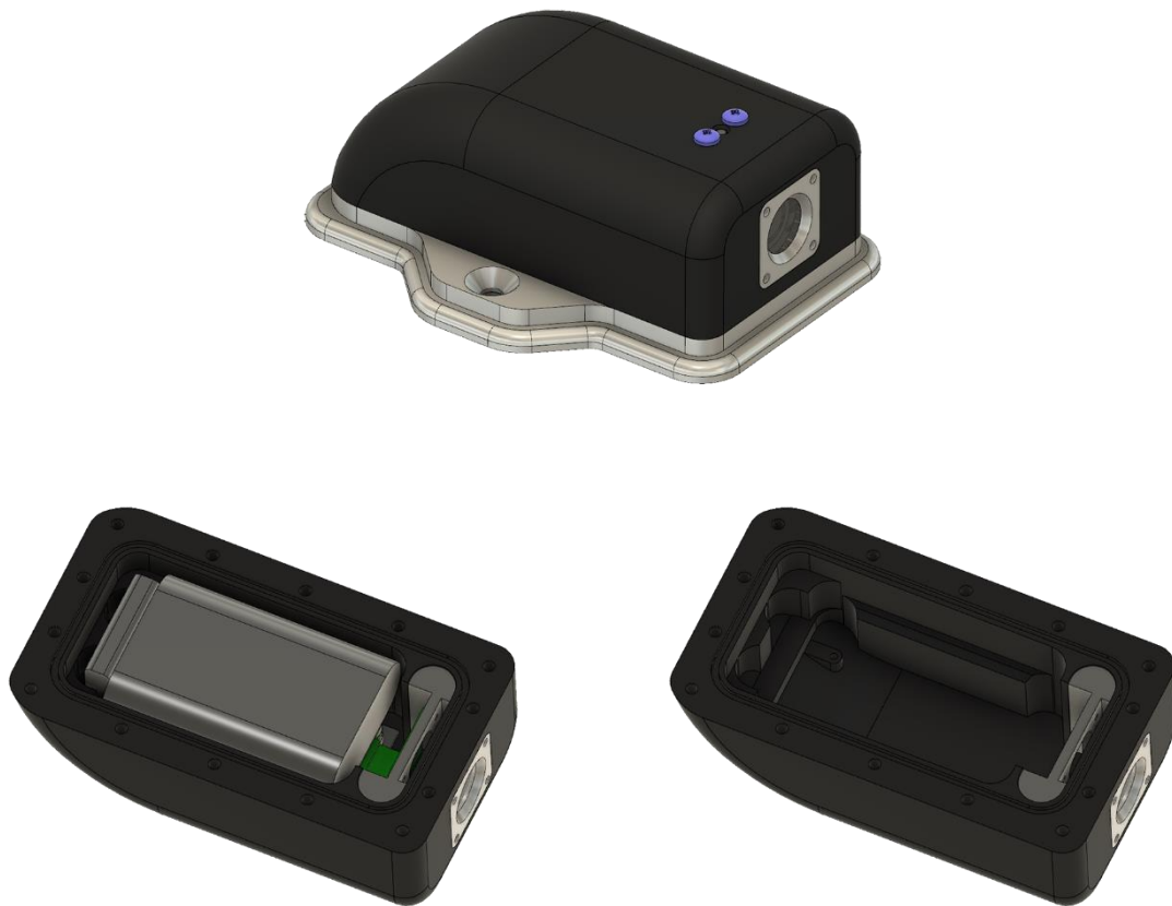
Figure 4.8: A few screenshots of the final version of PitStop Camera Tag in Autodesk Fusion 360. On the top is the assembled tag and on the bottom the inside of the enclosure with the mounting points for the electronic modules.
