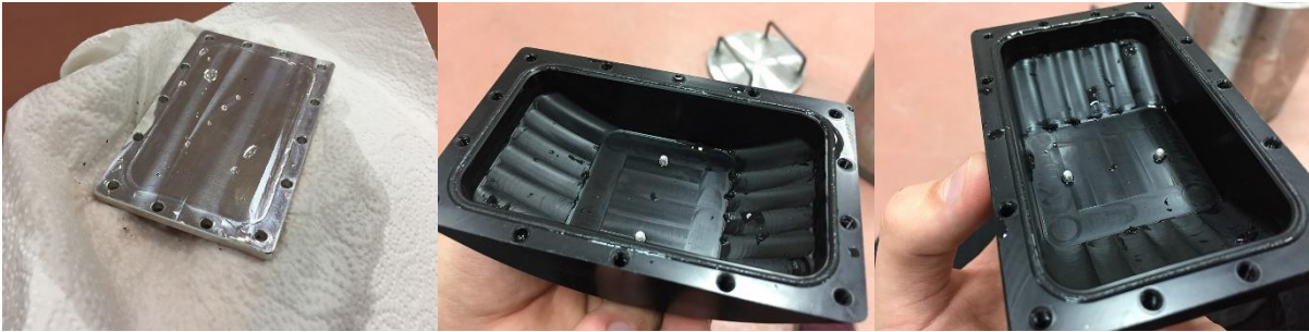
Figure 6.8: Polyoxymethylene (POM) enclosure shell with foamed polyurethane O-ring string was wet on the inside and on the lid. When the case was disassembled the water was flowing out, so it can be assumed that there was a lot of water inside.
