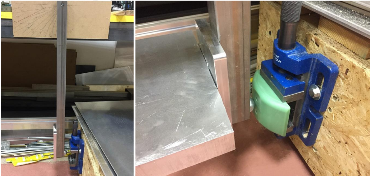
Figure 6.1: A pendulum like construction that was used to test the endurance of different turtle tag enclosures.
