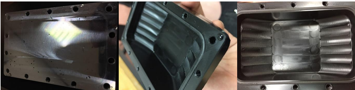
Figure 6.9: Polyoxymethylene (POM) enclosure shell with rubber O-ring string was the only combination that stayed completely dry. For this test there were no self-sealing screws for the salt water switch on the top of the case.
