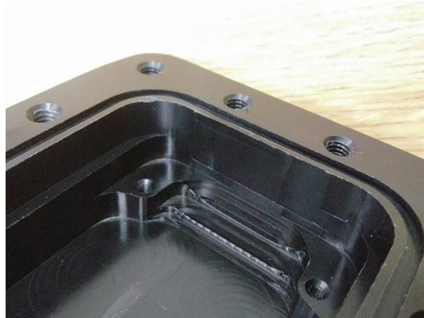
Figure 6.19: The turtle tag enclosures with the depth of O-ring groove of less than 1,25 mm had some problems with the deformations and damages on the enclosures.
