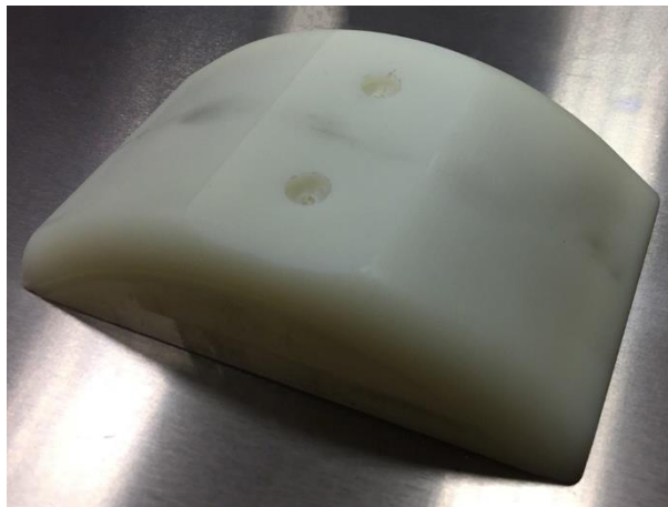
Figure 6.5: Polyamide 6 (PA6) enclosure shell tested wouldn't break even under the maximal load.
