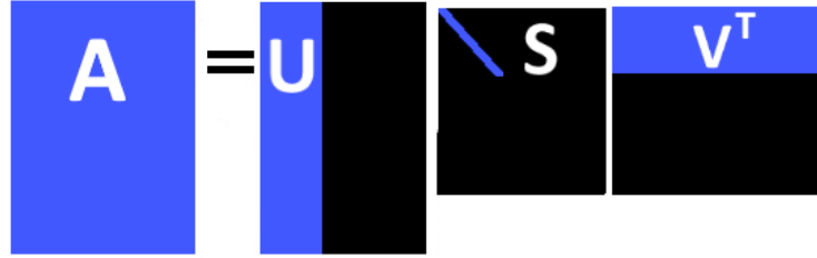
FIGURE 6.1: Decomposition of input matrix \mathbf{A} into diagonal matrix of singular values \mathbf{S} and matrices of left and right singular vectors. Light color illustrates low-rank approximation.
