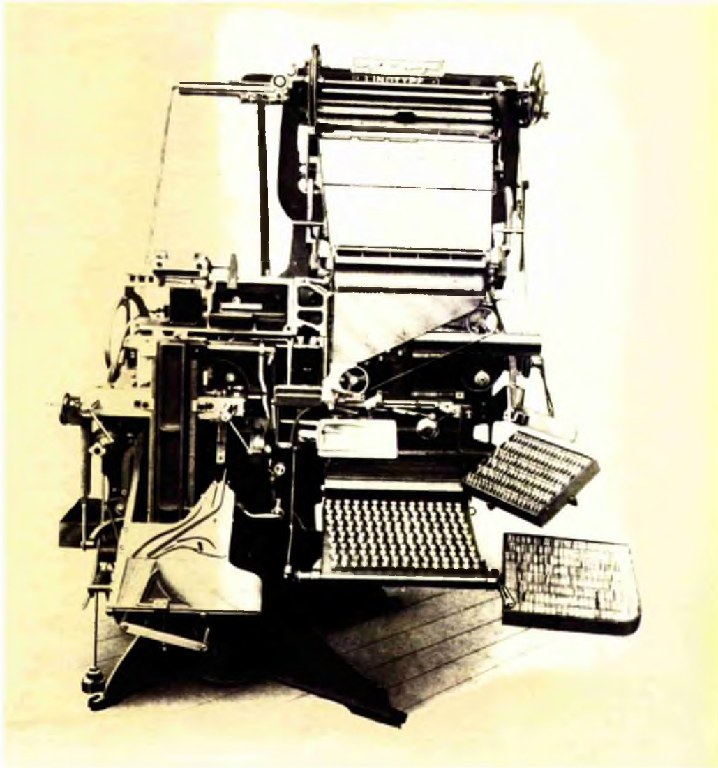
119. Fig. 1. Linotype Blower of 1886 Fig. 2. Linotype Arabic machine (Legros and Grant, Printing-Surfaces , figs. 401 and 407)
