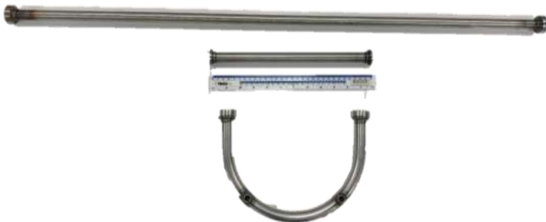
Fig. 6.7 Different optical path design, 1m and 30 cm straight optical path, 30 cm curved optical path
