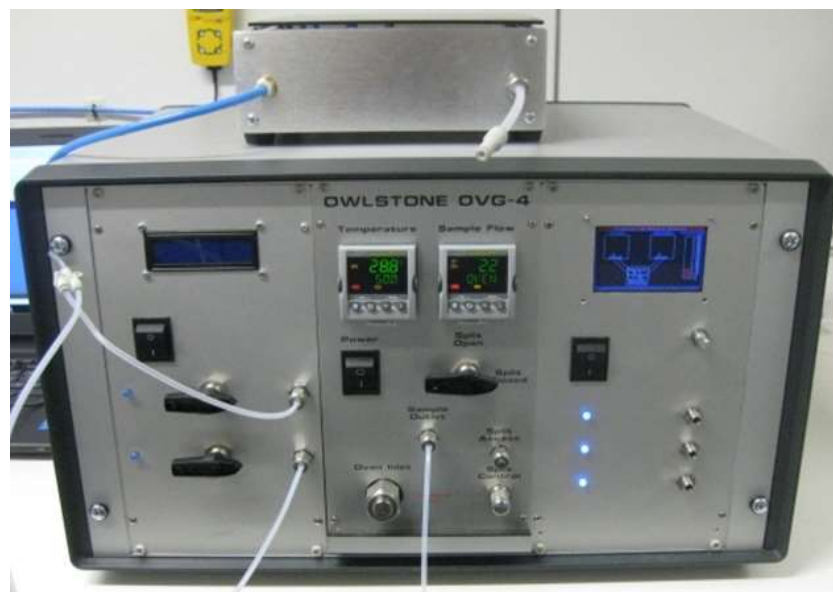
Fig. 5.15 Gas rig system with gas analyser on top of it
