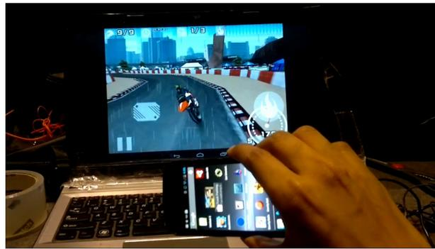
**Fig. 8.1.1 Snapshot 1 - Emulated Accelerometer in action**
