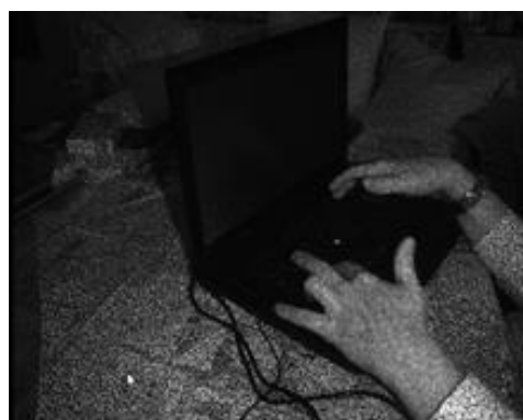
Figure 3. Infrared image shows the laser grid Kinect uses to calculate depth /2/
