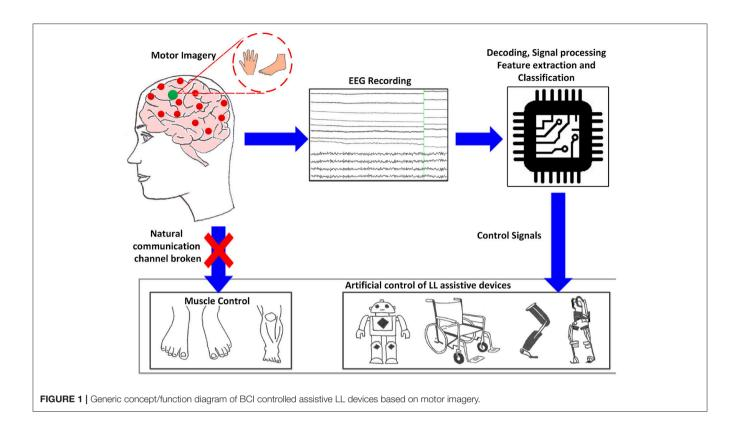
shows a schematic description of a BCI system based on MI, adapted from He et al. (2015). The user performs MI of limb(s), which is encoded in EEG reading; features representing the task are deciphered, processed and translated to commands in order to control assistive-robot device.
