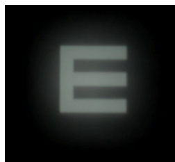
Fig. 3. Visualization 1 shows a through-focus video of a Sloan E when simulating a bifocal equal energy (50/50) design, when vergence changed from 0.5 D to -3.5 D at a temporal frequency of 50 Hz.
