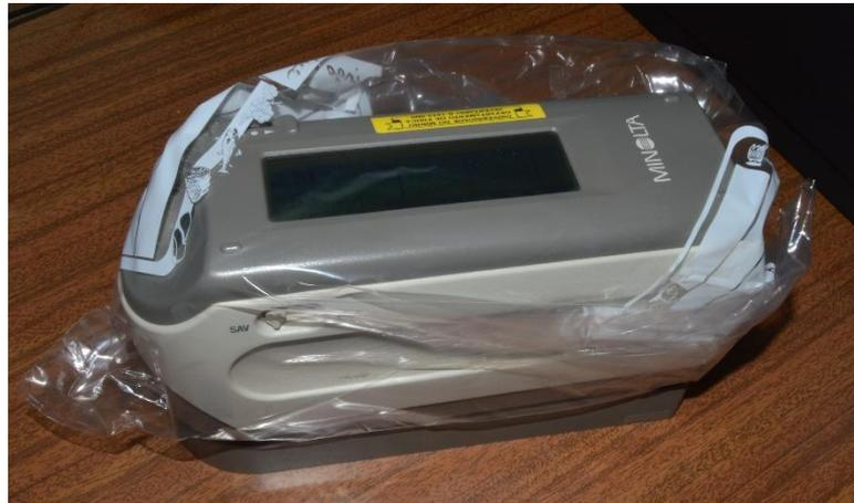
Figure 4.2. Contact spectrophotometer (CM-2600D, Konica Minolta, Japan) used for measuring dermatological patients. For biological protection it was repacked with a new plastic protector for every new patient. The transparent plastic covered the measure sensor at the bottom of the instrument and therefore its calibration had to be made having the plastic in account.
