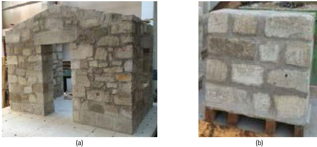
Figure 5.17 Stone masonry: (a) U-shape full-scale prototype, and (b) square wallets
