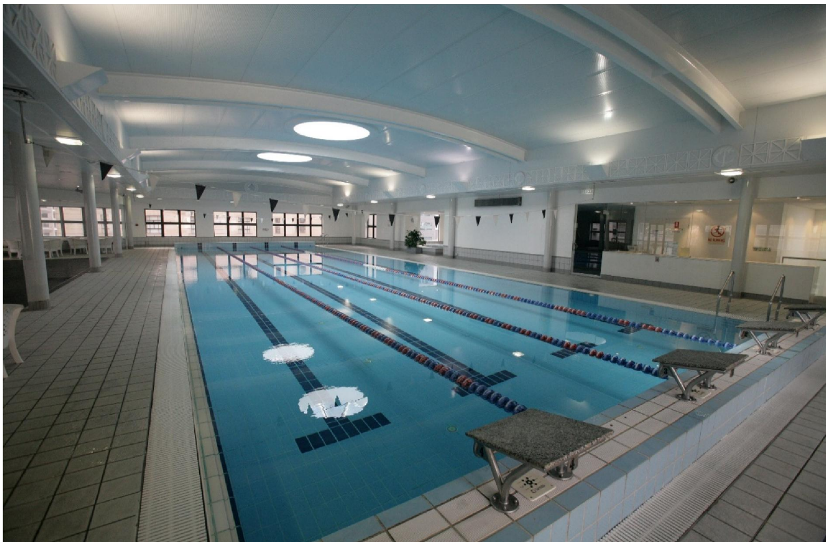
Fig. 51. The new swimming pool, located on the seventh floor just above the gymnasium and Health Centre. Built to strict International Olympic Committee standards, it was the highest suspended swimming pool in the Southern Hemisphere at the time. (Photo: Rene Marcel, 1997).
