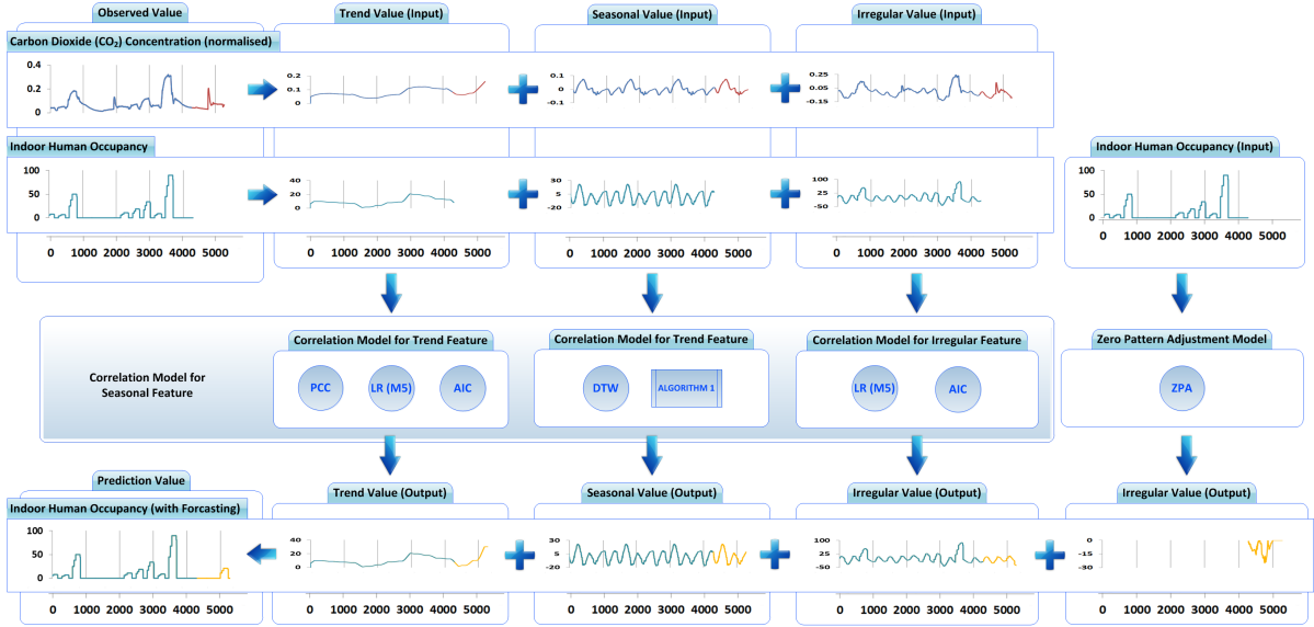
Figure 4.9: Large Room Utilisation Prediction (RUP) with Carbon Dioxide Sensor.
