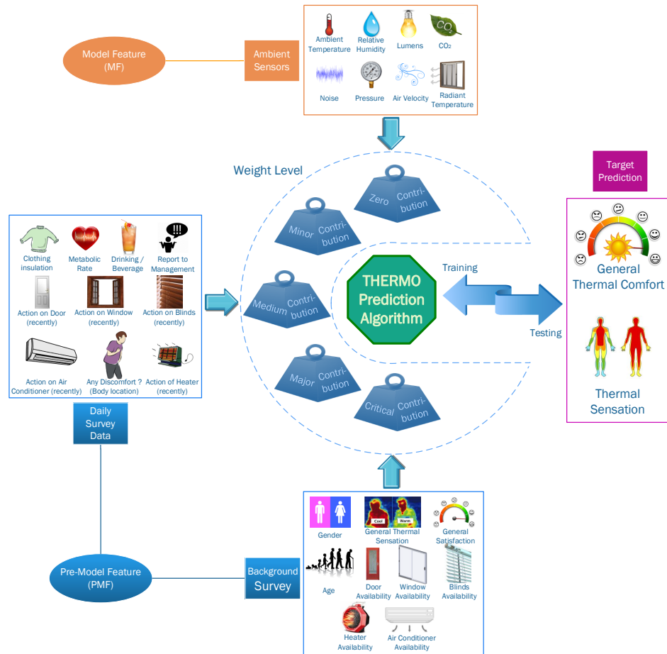
Figure 6.4: The data flow in THERMO and the detailed source of groups of features covering ambient sensors, daily survey data and background survey with the distribution of different weighted levels.
