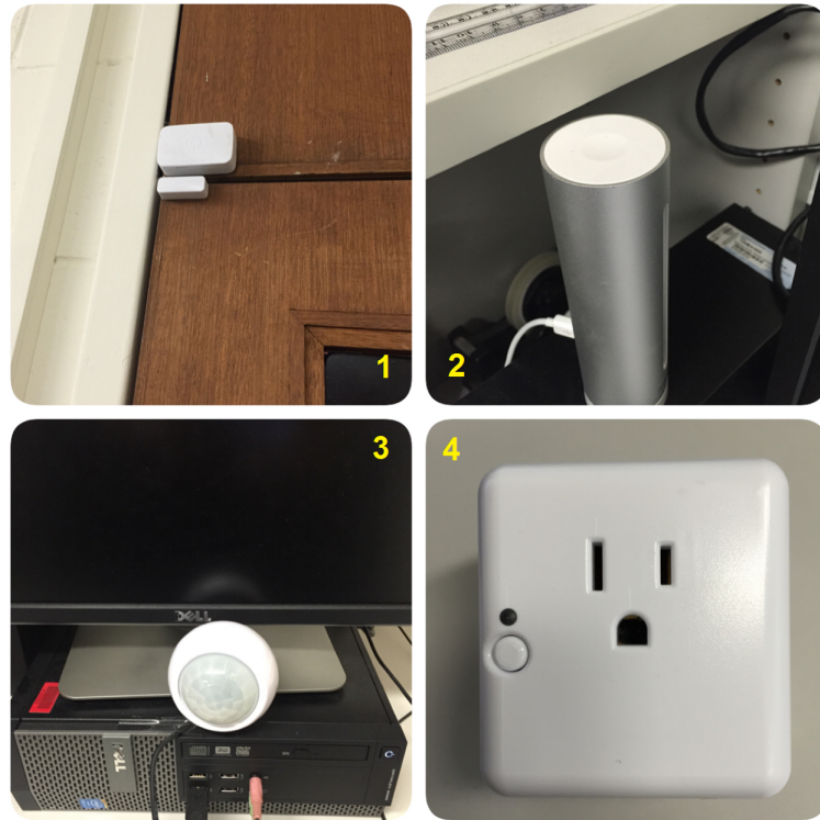
Figure 2.1: (1) SmartThings SmartSense Open/Closed Sensor; (2) Netatmo Urban Weather Station; (3) Z-Wave Aeon MultiSensor;(4) SmartThings SmartPower Outlet.
