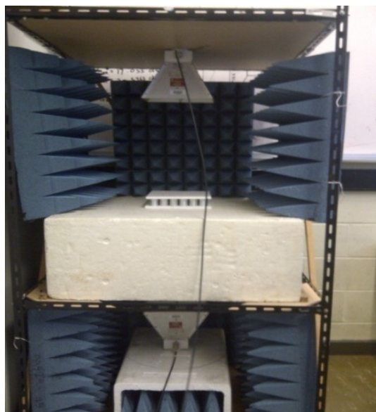
Figure 4.15: The measurement setup for 3-D Tapered FSS
