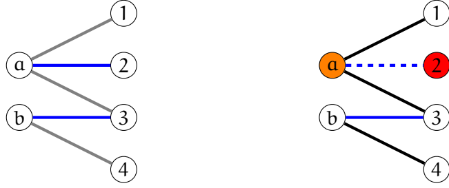
Figure 15: Key idea behind Algorithm 5. Input graph with \mathfrak{S} = W and the initial matching M (blue, on the left) and M -alternating paths from the "risky" job a to the remaining machines 1 and 2 after the failure of the machine 2 (on the right).
