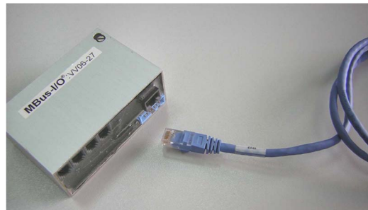
Fig. 7. MBus-I/O distributed electronic module for smart regulation of simple low-cost valves.
