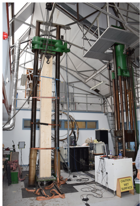
Figure 2: Amsler rig and one of the five largest ‘slender’ columns
