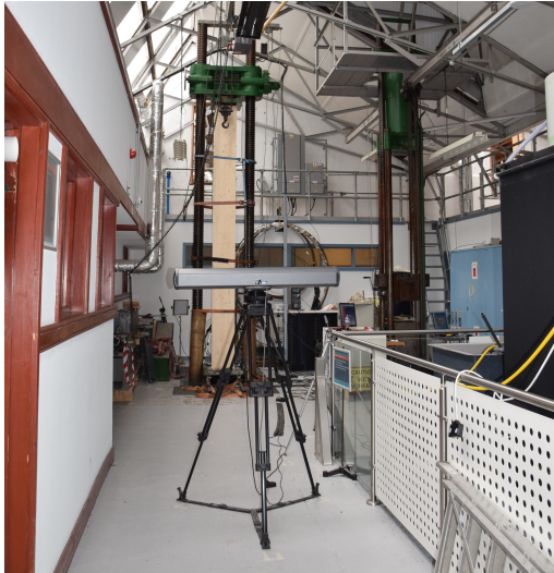
Figure 3: Test set up of the Optrax camera to record displacements
