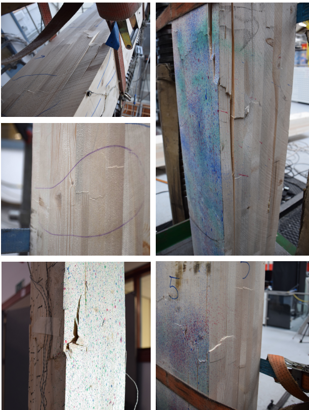
Figure 6: Failed samples showing kinkbands failures, failures through a knot and longitudinal splitting
