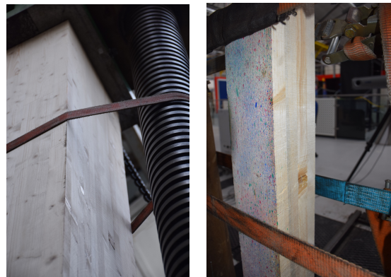
Figure 9: The ties in contact with a 360 sample (left) and not in contact with a 120 (right)
