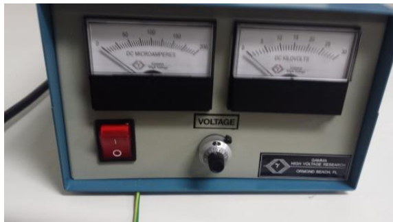
Figure 4.3 High voltage supply (Gamma High Voltage Research)
