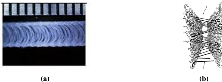
Figure 2.20: Spacer fabric (a) showing optical image (b) structural side view (adapted from Yip & Ng 2008)
