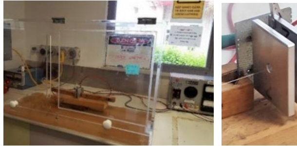
Figure 4.5 Setup used to extrude and pole polyvinylidene fluoride for validation
