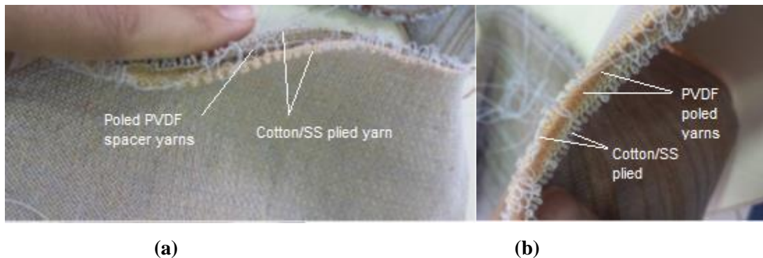
Figure 4.6: Spacer fabric prepared using poled yarns (a) front view (b)side view
