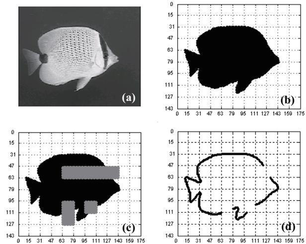
Fig. 3: (a) 1<sup>st</sup> frame of the *Bream* sequence. (b) Corresponding alpha plane of the *Bream*. (c) Received alpha plane with missing data. (d) Detected boundary for received alpha plane.
