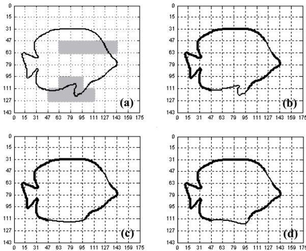
Fig. 6: (a) Shape contour of the 1<sup>st</sup> frame of the *Bream* sequence, the shaded blocks indicate the missing data. Concealment results using – (b) ISEC, (c) Bezier curve based technique [4], (d) Hermite spline based technique [5].
