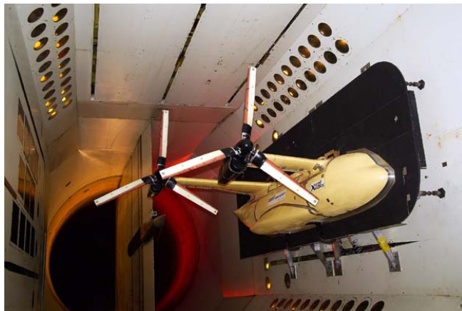
Figure 2.5: Boeing Quad Tilt-rotor Half-model in the Langley Wind Tunnel.
