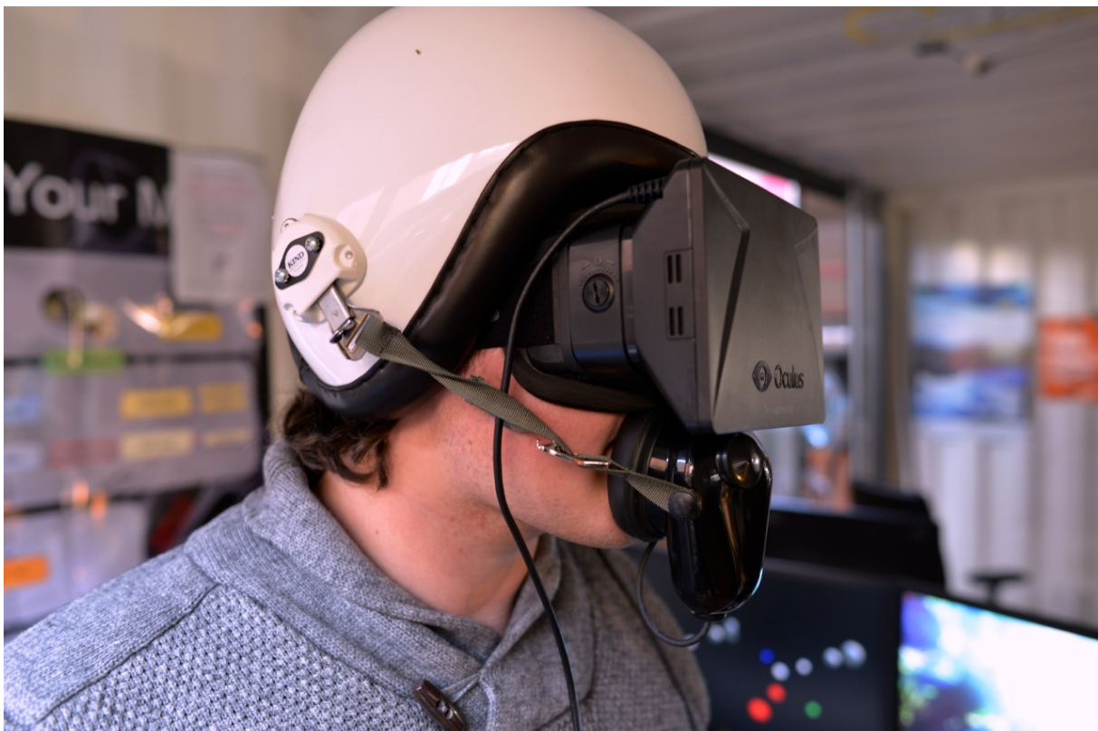
Figure 40 - Experimental setup of VR in combination with noise cancellation
