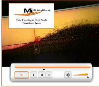
Figure 3: Still taken from a video made by MI HDD Mining and Waterwell. It shows fluid (yellow) moving up a pipe, entraining some particles (black) from the bed so they are suspended in the fluid.
