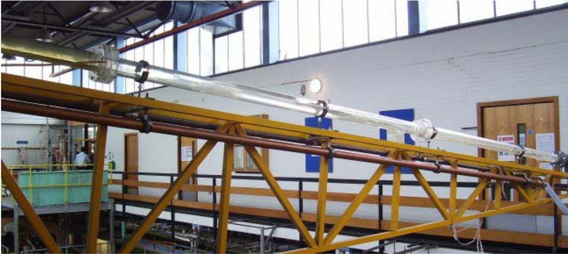
Figure 5: Barry Azzopardi's slug flow experimental facility at Nottingham University. A slug is travelling from right to left in the picture.
