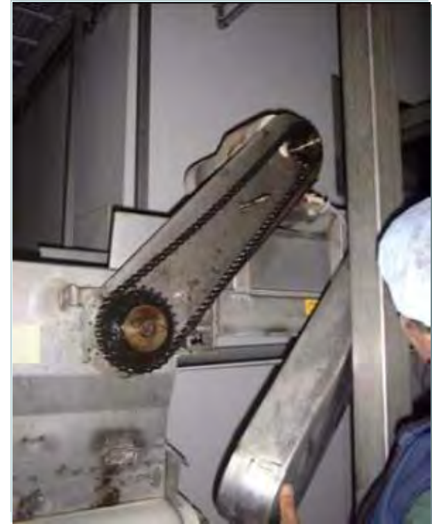
Open lubrication: Contamination risk
