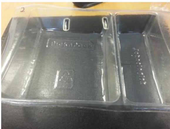
Figure 17 Tray made in a plaster mould from a 3-D printer
