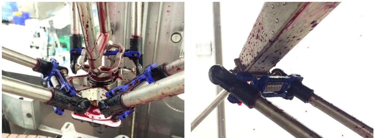
Fig. 42: Delta Robot after 1 minute of cleaning with the fixed nozzles.
