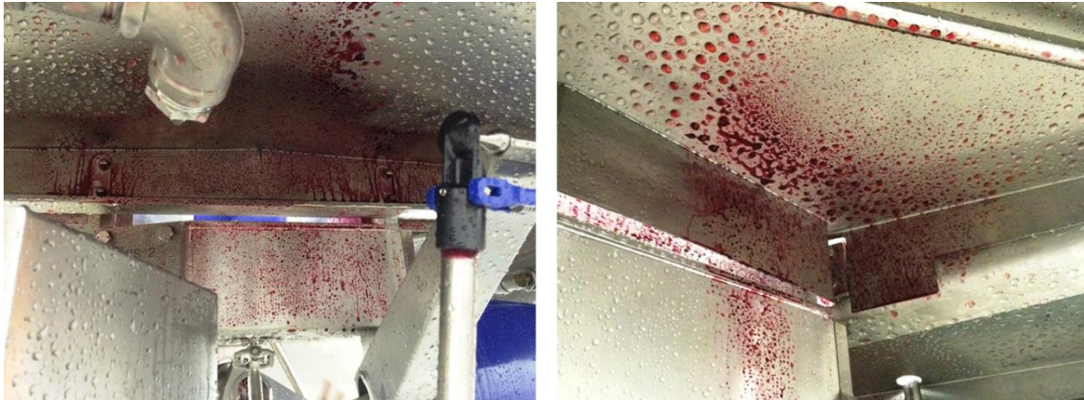
Fig. 49: Delta Robot after 20 minutes of cleaning with the fixed nozzles – spray shadows.
