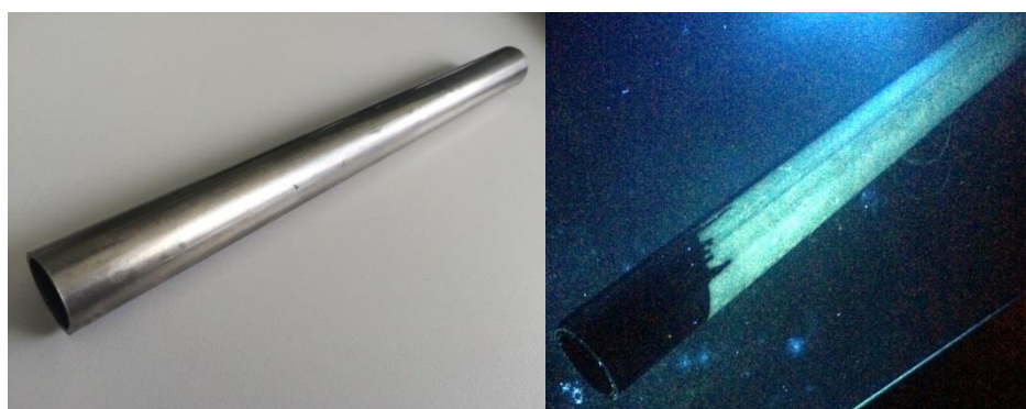
Fig. 5: Clean reference part (left) and reference part soiled with custard under UV light (right).
