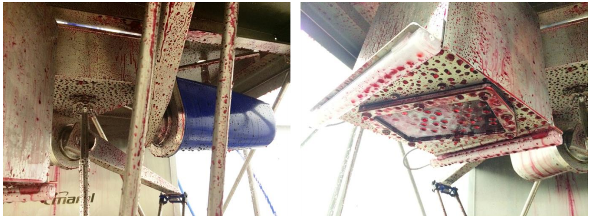
Fig. 41: Delta Robot after 1 minute of cleaning with the fixed nozzles.
