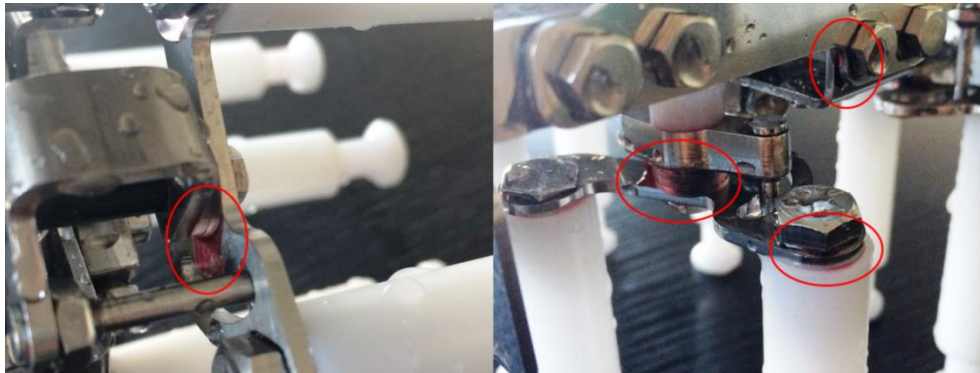
Fig. 8: Chicken gripper after Cleaning – Critical parts: Metal-to-metal-connections.
