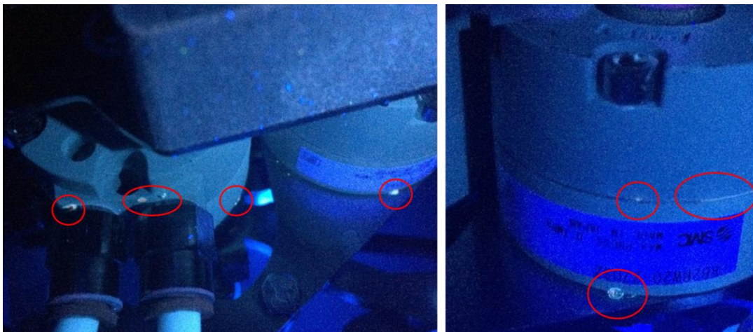
Fig. 22: Chicken gripper after 30 minutes of cleaning – Critical parts: Crevices.
