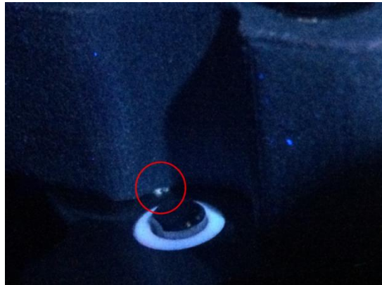
Fig. 24: Chicken gripper after 30 minutes of cleaning – Critical parts: Crevices.
