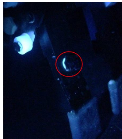
Fig. 35: Tomato Gripper after 3 minutes of cleaning – Critical parts: Metal-to-metal-connections.
