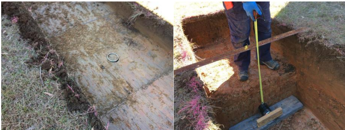
Figure 37. Photograph of sampler for intact materials for both (a) vertical cores (b) horizontal cores. Intact cores could only be obtained by this method for depths to ~1.1 m below ground level. Beyond this depth, the less-weathered shale materials fractured when trying to insert the steel corers.
