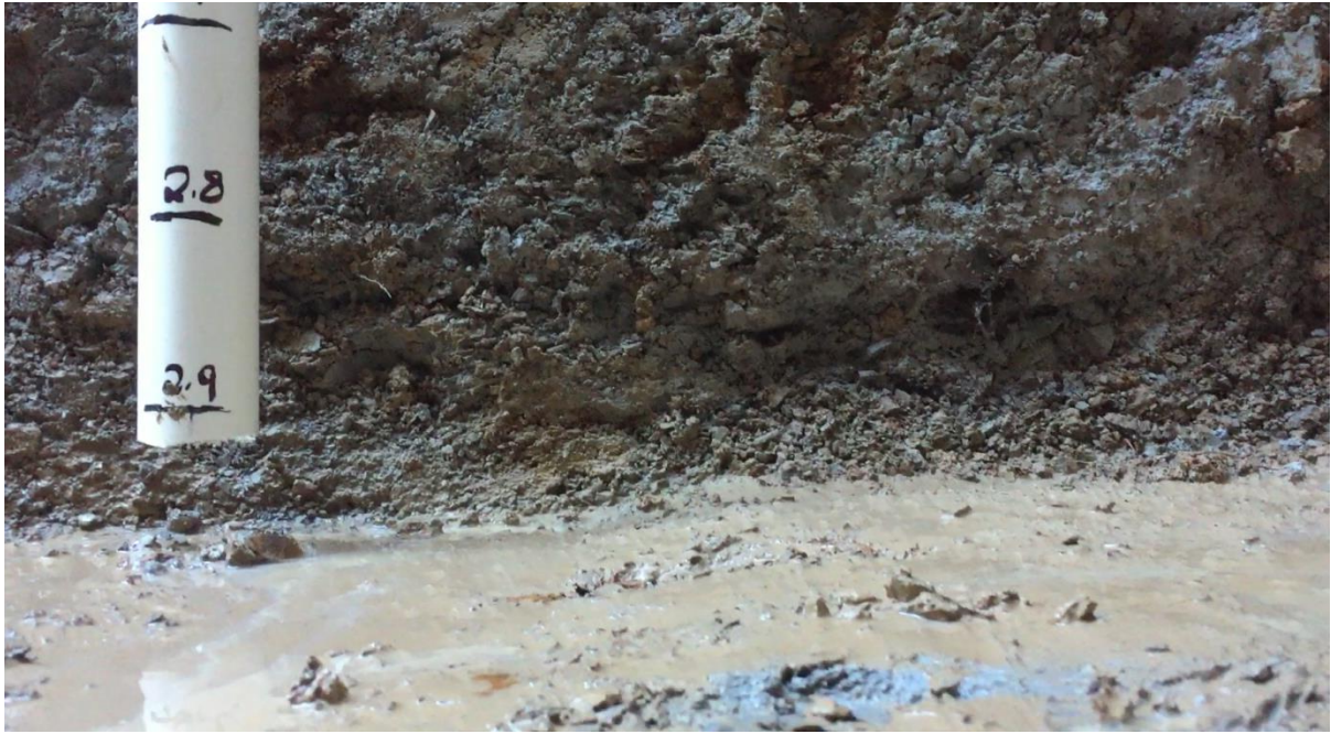
Figure 47. Video still of the base of the trench (southern trench face, western end). Note that the trench sides appear to be more weathered but less fractured at the western end and the nature of the connectivity appears different from that shown in Figure 46.
