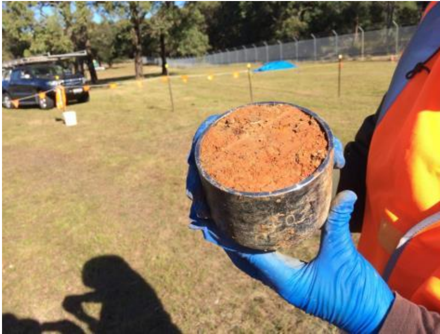
Figure 38. Example of intact core obtained from the red clay layer.
