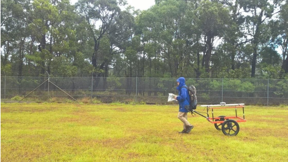
Figure 9. EM61 survey equipment over proposed test trench area.
