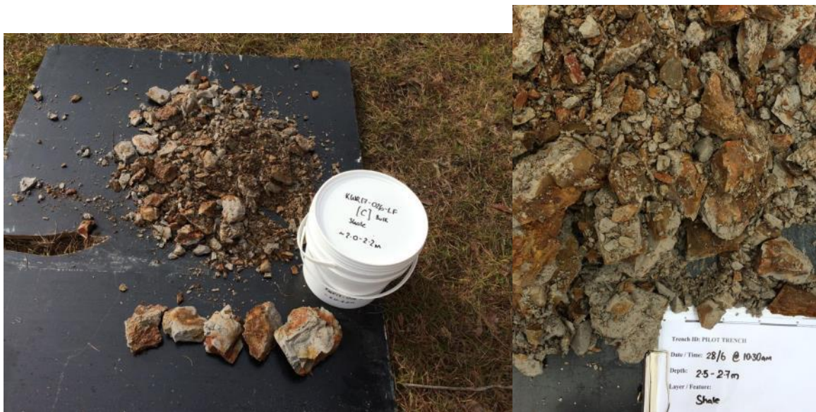
Figure 41. Examples of less weathered samples (a) from 2.0 – 2.2.m and (b) from 2.5 to 2.7 m.
