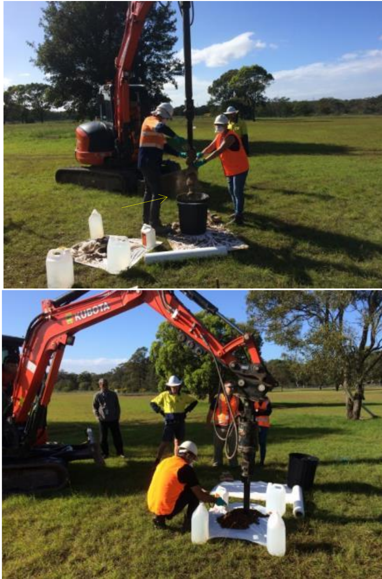
Figure 18. (a) Preliminary augering to ascertain absence of local contamination. Note the puff of dust (LHS). This shows how dry the shaly-clay layer is, despite several weeks of prior rainy weather. (b) Sampling from auger. External gamma screening on all samples revealed no contamination above background
