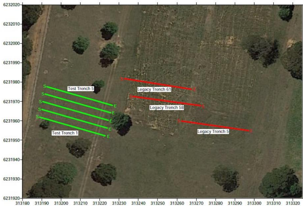
Figure 12. Close-spaced resistivity survey lines showing the legacy trench area (red) and the proposed experimental test trench areas (green).
