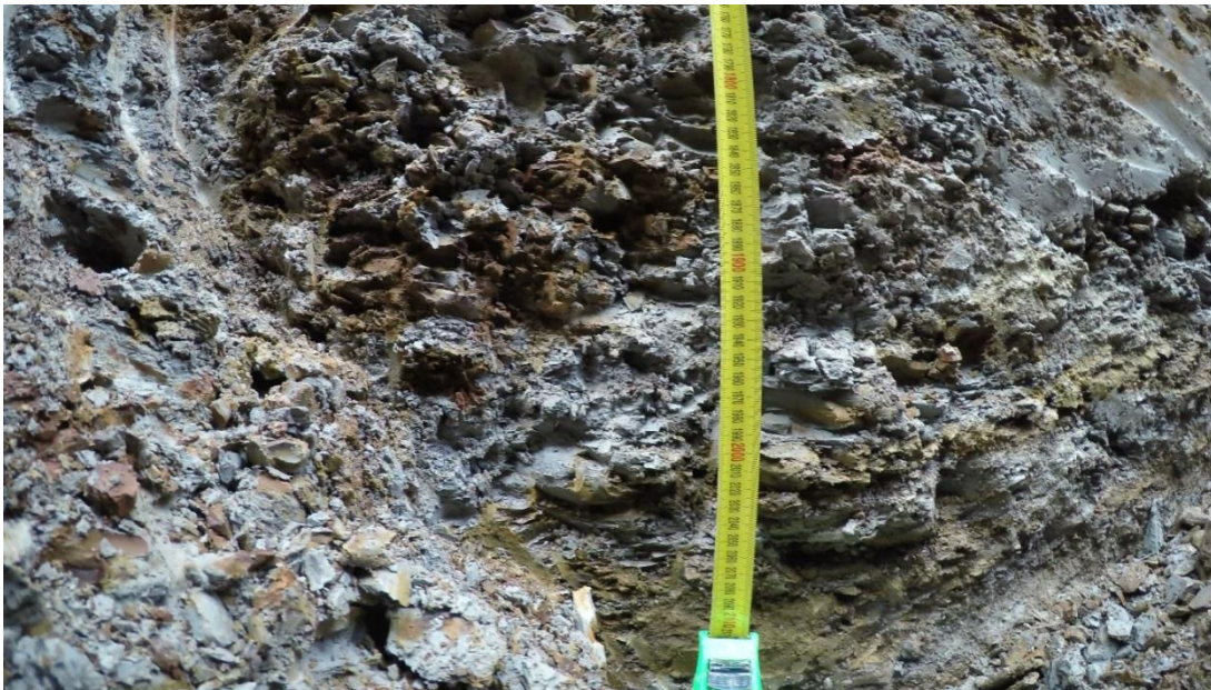
Figure 52. Weathered shale layer (~1.7-2.0 m) immediately above a seepage accumulation zone (northern face of trench).
