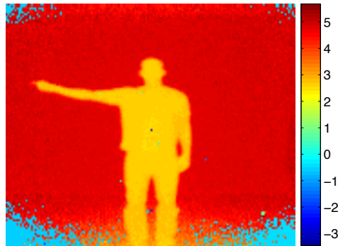
Figure 2.6: Depth image obtained by the active laser-based SwissRanger ® SR2 time of flight sensor with the depth values represented by pixel color (image from Holte et al., 2008).
