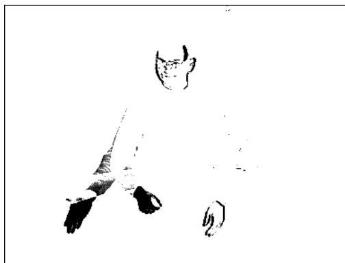
Figure 3.4: Result image obtained by performing ‘background’ subtraction. Note the two left hands resulting from the difference between the background hand position and the current hand position.
