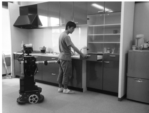
Figure 1.2: The robot Robovie supporting a human in the kitchen by giving verbal and gestural advice on the presumed next action (image from Fukuda et al., 2005).
