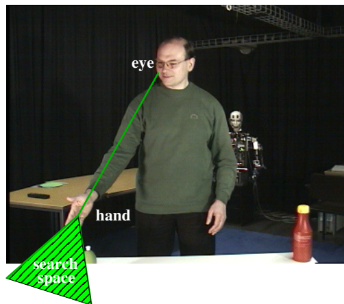
Figure 6.2: Using body posture information to create an eye-hand line that restricts the search space for object search.
