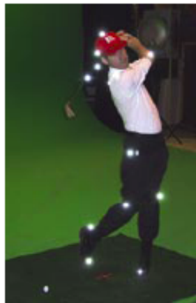
Figure 2.3: The highlighted dots are infrared reflections from markers attached to the human body and golf club.
