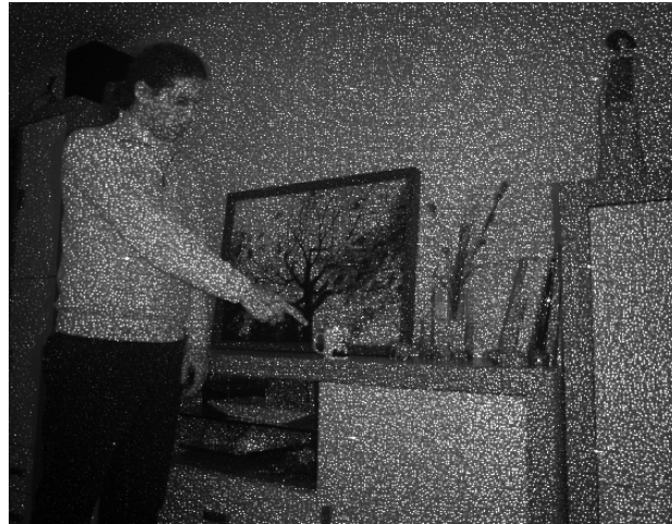
Figure 2.7: Image from Kinect sensor exhibiting pattern of structured infrared light.
