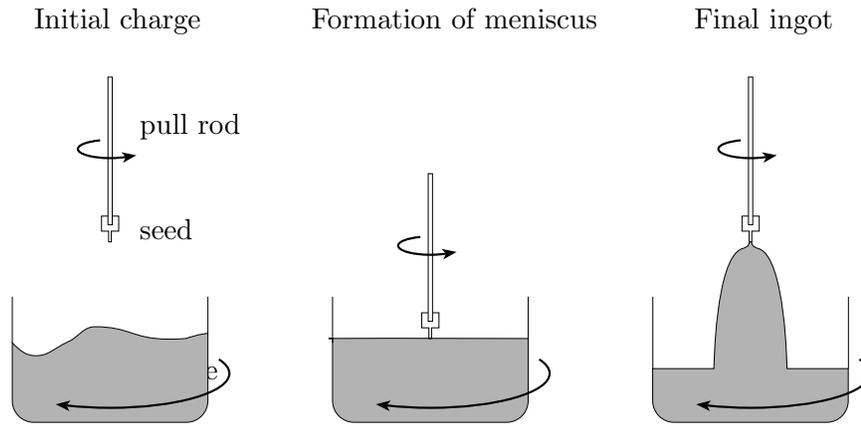
Figure 2.1: The Czochralski crystal pulling technique.
