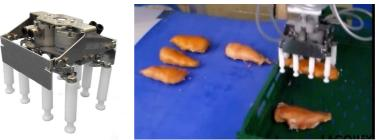
Figure 21 Pneumatic gripper
