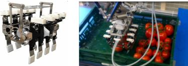
Figure 20 Electrical gripper
