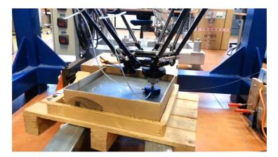
Figure 10: Test of dynamic behaviour for air bearings
