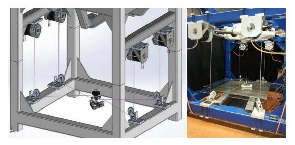
Figure 13: Test bench for the test of cables, drums and winch behaviour
