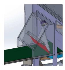
Figure 36: Integrated vision system into the frame of the robot
