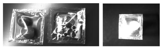
Figure 33: Diffuse light vs selected light (high intensity, red)
