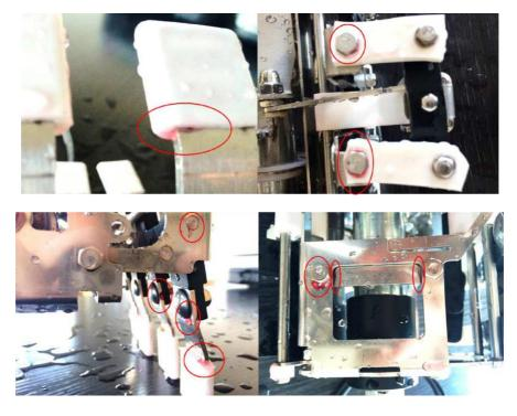
Figure 40: Tomato gripper after Cleaning
