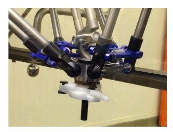
Figure 19 Fast gripper changer
