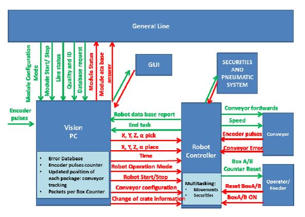
Figure 14: Internal and external communications of the cable robot module
