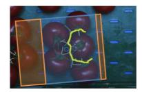
Figure 28 – An illustration of the gripper placed on the vine. The blue circles form the pinch gripper. The small orange rectangle is the row of closed fingers and the larger orange rectangle is the row of open fingers. When opened, the fingers do not collide with other vine tomatoes.
