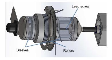
Figure 3: Detailed view of winch
