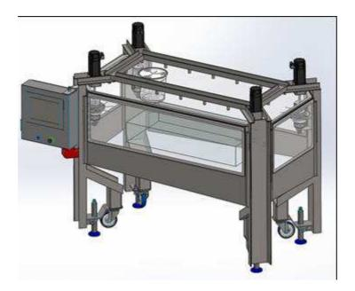
Figure 1: General view of cable robot
