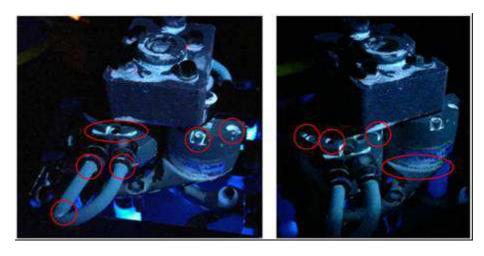
Figure 41: Chicken gripper after 3 minutes of cleaning
