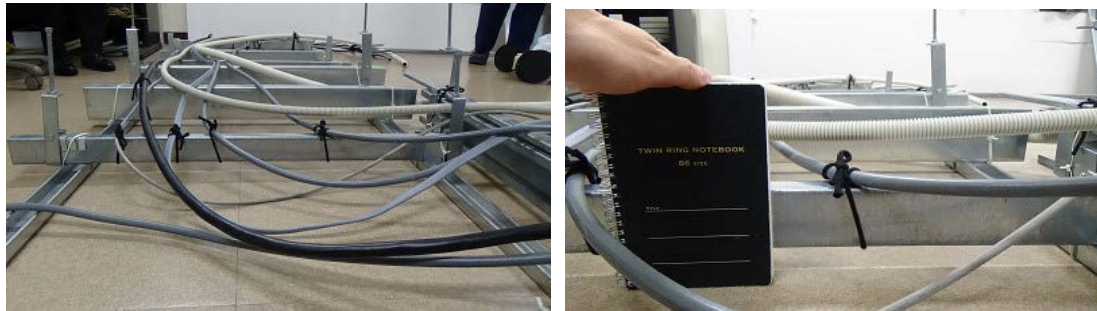
(a) Steps due to reinforcing bars and cables (b) Comparison of size with B6 size notebook
