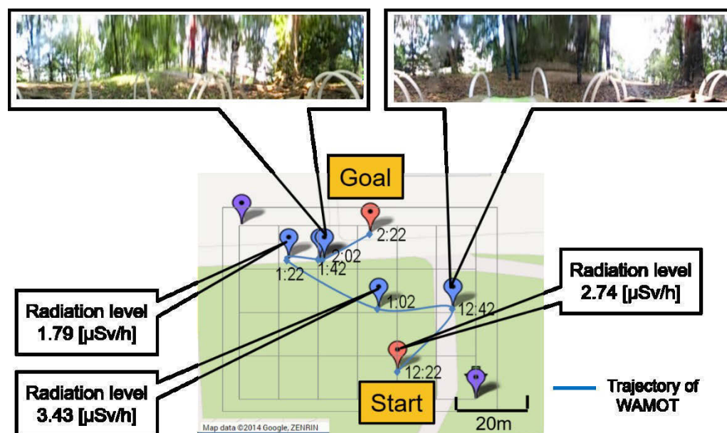
Figure 4.11 Trajectory of WAMOT: The robot starts from the starting point (12:22) and finish on goal point (2:22).
