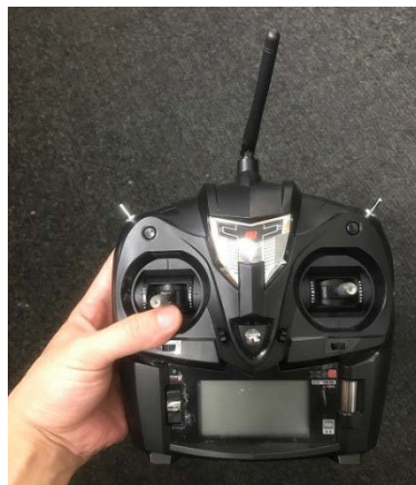
Figure 4.33 Transmitter used in teleoperation system
