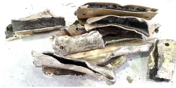
Figure 4-16: Al particles with glass and sealant.
