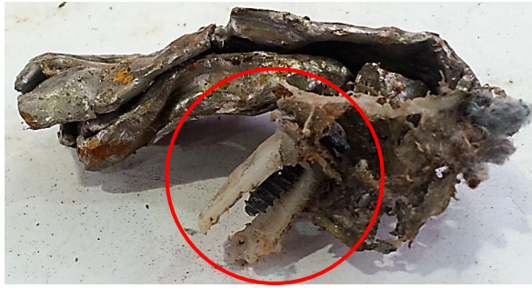
Figure 4-11: Steel particle with plastic rivet.
