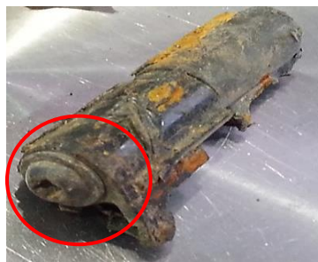
Figure 4-20: Particle with steel screw encapsulated in plastic.
