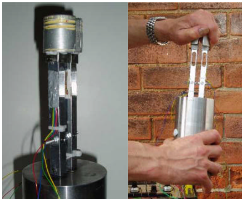
Figure 12: the grip gauge with the 30x35 extra deep ROPP closure attachment on the left and an illustration of how it is used on the right.
