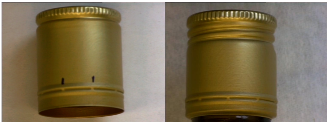
Figures 3a and 3b: showing closure before and after application respectively
