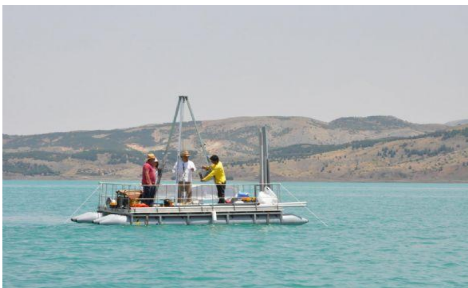
Figure 2.2 : Core sampling on a portable platform of ITU EMCOL.
