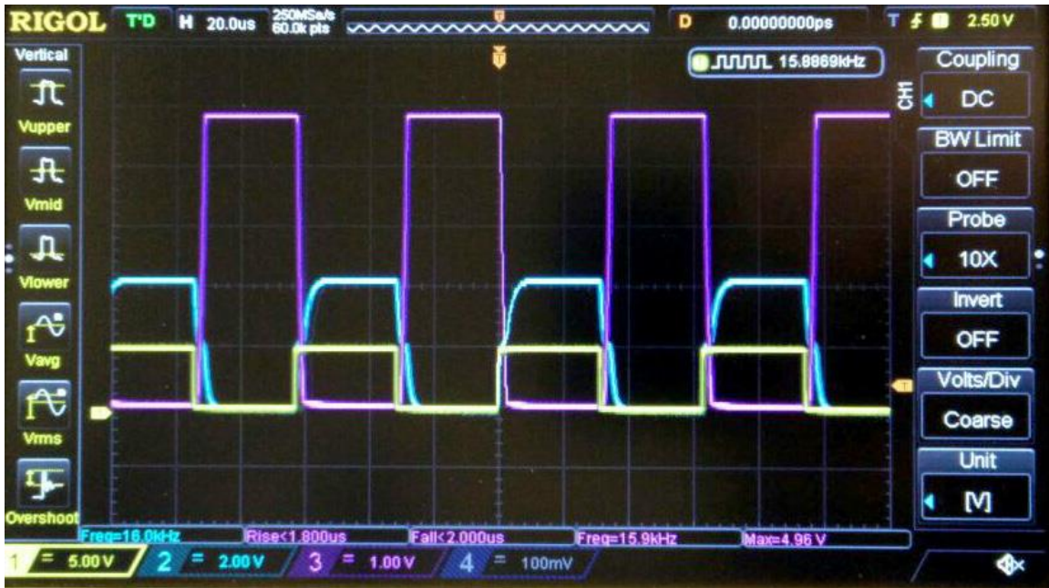
Figure 58. Output of the driver circuit
