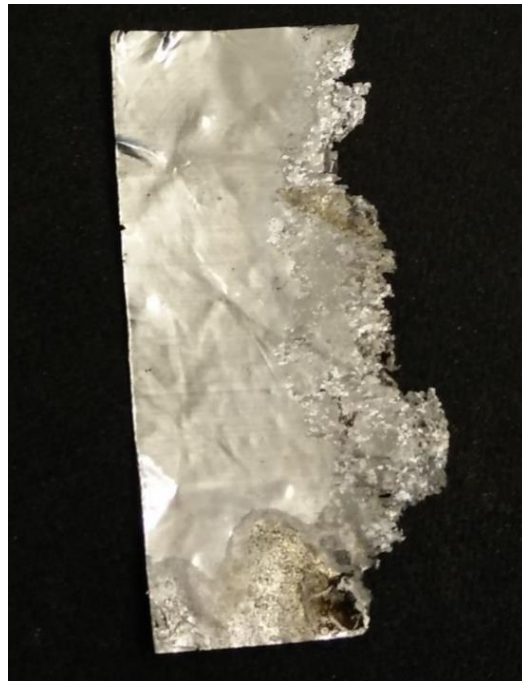
Figure 62. A 20-micron aluminum thin foil after applying the brazing flux for the minimum amount of recommended time
