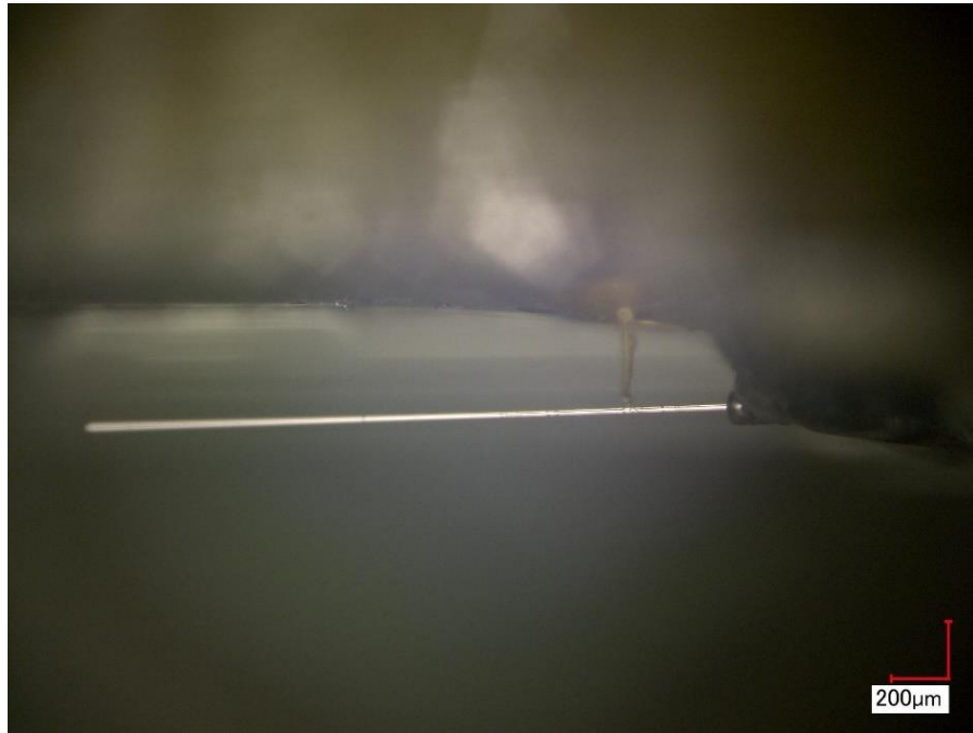
Figure 37. A 20-micron brass sample with a 15-micron optical fiber on a PCB in a perpendicular set up
