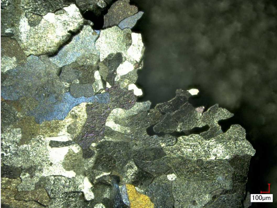
Figure 63. A 20-micron aluminum foil after applying the brazing flux for the recommended time
