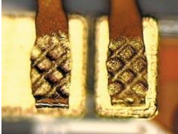
Figure 61. 25-micron wide copper ribbon cable bonded to a gold pad inside of a hard drive
